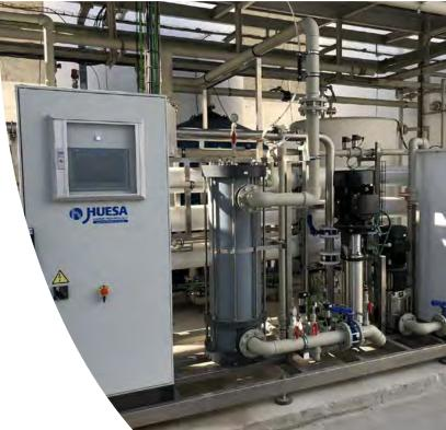
Ultrafiltration is a membrane technology that takes place within a membrane porosity range between 0.001 and 0.1  $\mu$ m. It is used for the selective removal of suspended matter, particulate matter, large macromolecules, colloidal matter or microorganisms.
