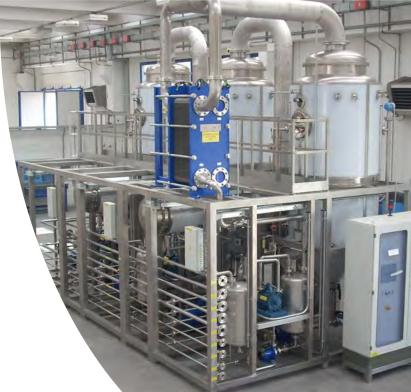
Advanced oxidation processes (AOP's) are physical-chemical processes capable of producing changes in the structure of pollutants by increasing their biodegradability through the use of the hydroxyl radical (OH-).
