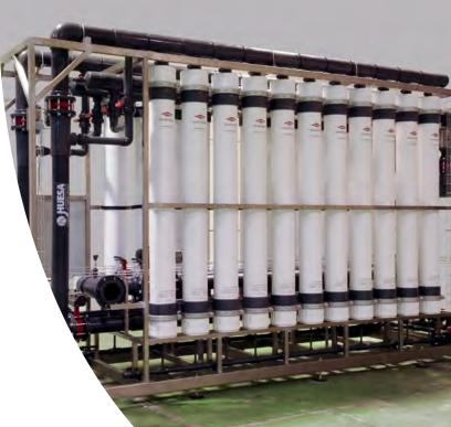
Nanofiltration is a membrane filtration process that takes place in a porosity range between 150-500 Dalton, which achieves, among others, the separation of polyvalent ions with an effectiveness of more than 95 %, as well as organic matter of low molecular weight (sugar, proteins, etc.).
