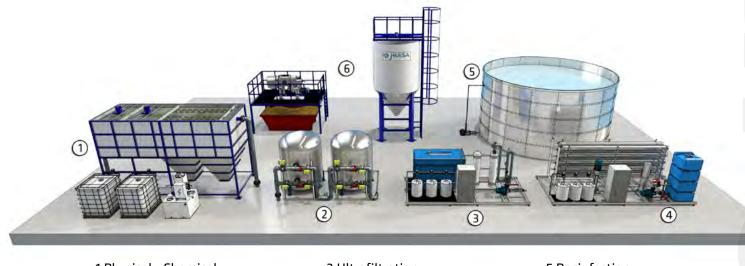
1 Physical - Chemical 2 Filtration 3 Ultrafiltration 4 Reverse Osmosis 5 Desinfection 6 Sludge Treatment Water is widely used in industry and is rarely found in the right conditions for direct incorporation into the process. The quality requirements vary according to the industrial activity, while water is used more or less extensively.
