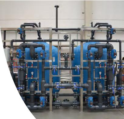
Filtration within a porosity zone between 0.1  $\mu$ m - 10  $\mu$ m, which allows the removal of suspended solids, fine particles, colloids, algae and microorganisms, among others.
